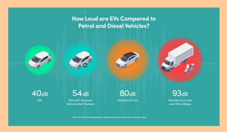
Electric vehicles are a lot quieter than conventional ones. So quiet, it's becoming mandatory in many areas around the world that they produce a sound to alert pedestrians to them. The EVs and hybrids must make a noise above 56dB when a vehicle is 12mph and under using an acoustic vehicle alert system (AVAS). EVs are much quieter compared to petrol and diesel as they don't have a combustion engine. This means the only sound they generate is from the tyres on the road and the wind resistance.
