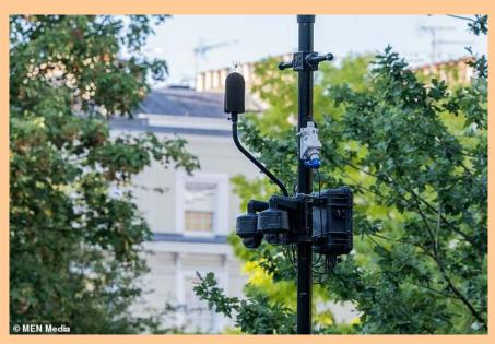
The cameras, which are triggered by a number of microphones, can pinpoint vehicles exceeding the 74-decibel legal limit as they pass by. Pictures of vehicle numberplates together with recordings of the vehicle noise are then used by local police to identify and fine drivers. Trials took place in Bradford, Great Yarmouth, Birmingham and South Gloucestershire near Bristol.
